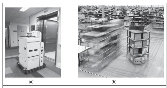
**Figure 25.27** (a) The Helpmate robot transports food and other medical items in dozens of hospitals worldwide. (b) Kiva robots are part of a material-handling system for moving shelves in fulfillment centers. Image courtesy of Kiva Systems.
