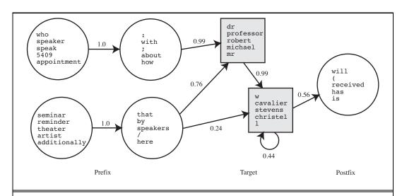
**Figure 22.2** Hidden Markov model for the **speaker** of a talk announcement. The two square states are the target (note the second target state has a self-loop, so the target can match a string of any length), the four circles to the left are the prefix, and the one on the right is the postfix. For each state, only a few of the high-probability words are shown. From Freitag and McCallum (2000).
