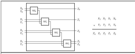
**Figure 8.8** A four-bit adder. Each  $Ad_i$  is a one-bit adder, as in Figure 8.6 on page 309.
