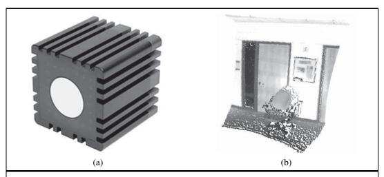
**Figure 25.3** (a) Time of flight camera; image courtesy of Mesa Imaging GmbH. (b) 3D range image obtained with this camera. The range image makes it possible to detect obstacles and objects in a robot's vicinity.
