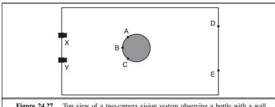
**Figure 24.27** Top view of a two-camera vision system observing a bottle with a wall behind it.
