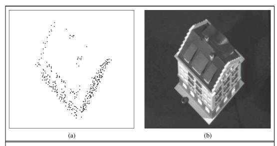
**Figure 24.19** (a) Three-dimensional reconstruction of the locations of the image features in Figure 24.18, shown from above. (b) The real house, taken from the same position.
