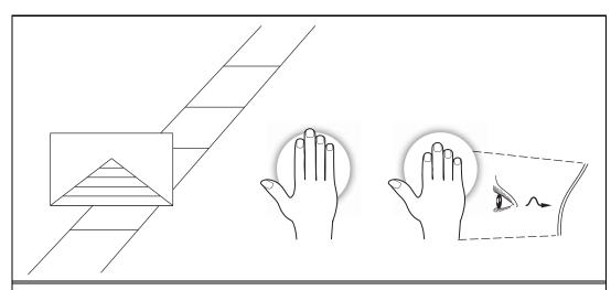
**Figure 24.1** Imaging distorts geometry. Parallel lines appear to meet in the distance, as in the image of the railway tracks on the left. In the center, a small hand blocks out most of a large moon. On the right is a foreshortening effect: the hand is tilted away from the eye, making it appear shorter than in the center figure.
