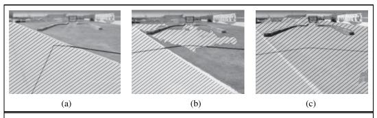
**Figure 25.13** Sequence of "drivable surface" classifier results using adaptive vision. In (a) only the road is classified as drivable (striped area). The V-shaped dark line shows where the vehicle is heading. In (b) the vehicle is commanded to drive off the road, onto a grassy surface, and the classifier is beginning to classify some of the grass as drivable. In (c) the vehicle has updated its model of drivable surface to correspond to grass as well as road.
