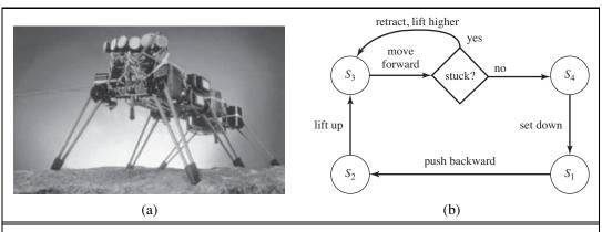
**Figure 25.24** (a) Genghis, a hexapod robot. (b) An augmented finite state machine (AFSM) for the control of a single leg. Notice that this AFSM reacts to sensor feedback: if a leg is stuck during the forward swinging phase, it will be lifted increasingly higher.
