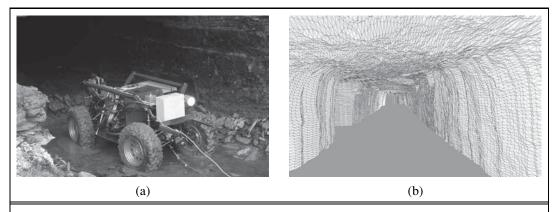
**Figure 25.29** (a) A robot mapping an abandoned coal mine. (b) A 3D map of the mine acquired by the robot.
