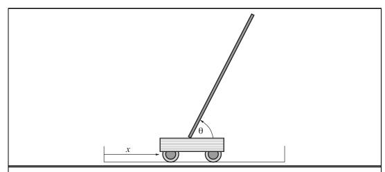
**Figure 21.9** Setup for the problem of balancing a long pole on top of a moving cart. The cart can be jerked left or right by a controller that observes x,  $\theta$ ,  $\dot{x}$ , and  $\dot{\theta}$ .
