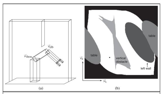
**Figure 25.14** (a) Workspace representation of a robot arm with 2 DOFs. The workspace is a box with a flat obstacle hanging from the ceiling. (b) Configuration space of the same robot. Only white regions in the space are configurations that are free of collisions. The dot in this diagram corresponds to the configuration of the robot shown on the left.
