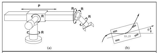
**Figure 25.4** (a) The Stanford Manipulator, an early robot arm with five revolute joints (R) and one prismatic joint (P), for a total of six degrees of freedom. (b) Motion of a nonholonomic four-wheeled vehicle with front-wheel steering.
