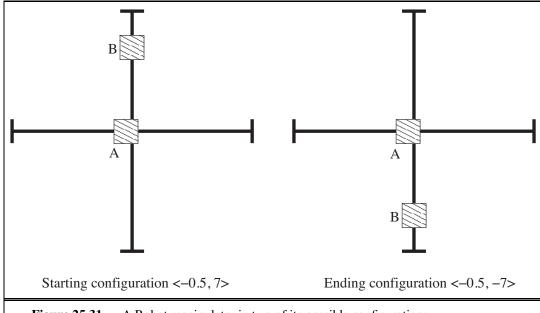
**Figure 25.31** A Robot manipulator in two of its possible configurations.
