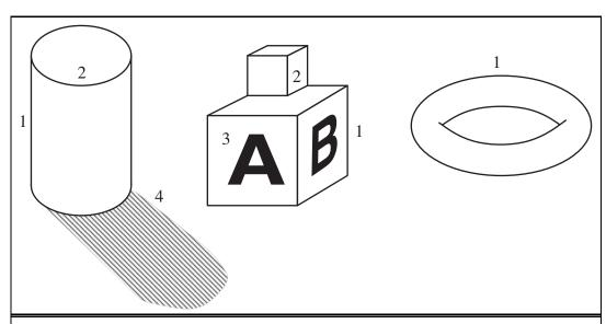
**Figure 24.6** Different kinds of edges: (1) depth discontinuities; (2) surface orientation discontinuities; (3) reflectance discontinuities; (4) illumination discontinuities (shadows).
