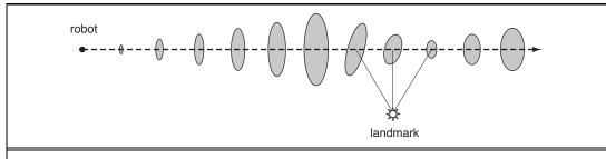
**Figure 25.12** Example of localization using the extended Kalman filter. The robot moves on a straight line. As it progresses, its uncertainty increases gradually, as illustrated by the error ellipses. When it observes a landmark with known position, the uncertainty is reduced.
