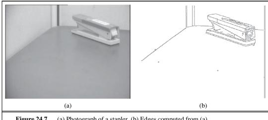
Figure 24.7 (a) Photograph of a stapler. (b) Edges computed from (a).
