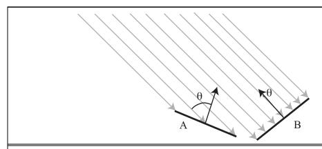
Two surface patches are illuminated by a distant point source, whose rays are Figure 24.5 shown as gray arrowheads. Patch A is tilted away from the source ( $\theta$  is close to  $90^{\circ}$ ) and collects less energy, because it cuts fewer light rays per unit surface area. Patch B, facing the source ( $\theta$  is close to  $0^0$ ), collects more energy.
