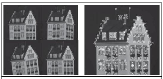
**Figure 24.18** (a) Four frames from a video sequence in which the camera is moved and rotated relative to the object. (b) The first frame of the sequence, annotated with small boxes highlighting the features found by the feature detector. (Courtesy of Carlo Tomasi.)
