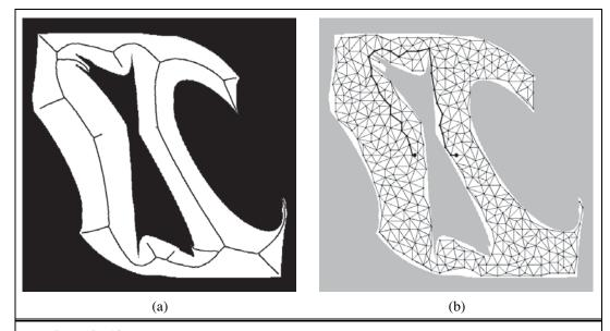
**Figure 25.18** (a) The Voronoi graph is the set of points equidistant to two or more obstacles in configuration space. (b) A probabilistic roadmap, composed of 400 randomly chosen points in free space.
