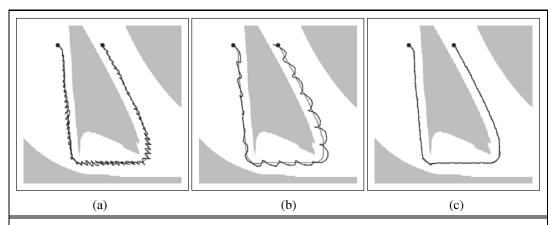
**Figure 25.22** Robot arm control using (a) proportional control with gain factor 1.0, (b) proportional control with gain factor 0.1, and (c) PD (proportional derivative) control with gain factors 0.3 for the proportional component and 0.8 for the differential component. In all cases the robot arm tries to follow the path shown in gray.
