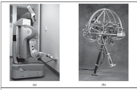
**Figure 25.5** (a) Mobile manipulator plugging its charge cable into a wall outlet. Image courtesy of Willow Garage, © 2009. (b) One of Marc Raibert's legged robots in motion.
