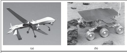
**Figure 25.2** (a) Predator, an unmanned aerial vehicle (UAV) used by the U.S. Military. Image courtesy of General Atomics Aeronautical Systems. (b) NASA's Sojourner, a mobile robot that explored the surface of Mars in July 1997.
