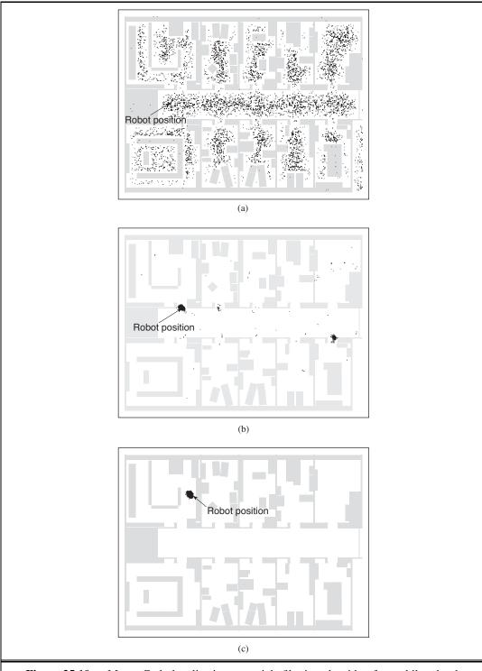
**Figure 25.10** Monte Carlo localization, a particle filtering algorithm for mobile robot localization. (a) Initial, global uncertainty. (b) Approximately bimodal uncertainty after navigating in the (symmetric) corridor. (c) Unimodal uncertainty after entering a room and finding it to be distinctive.
