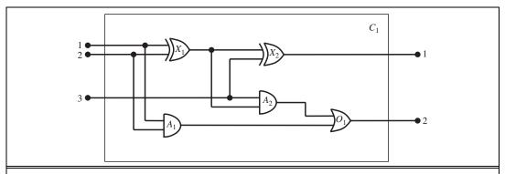
**Figure 8.6** A digital circuit C1, purporting to be a one-bit full adder. The first two inputs are the two bits to be added, and the third input is a carry bit. The first output is the sum, and the second output is a carry bit for the next adder. The circuit contains two XOR gates, two AND gates, and one OR gate.
