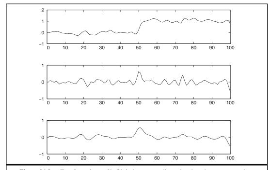
Figure 24.8 Top: Intensity profile I(x) along a one-dimensional section across an edge at x = 50. Middle: The derivative of intensity, I'(x). Large values of this function correspond to edges, but the function is noisy. Bottom: The derivative of a smoothed version of the intensity,  $(I*G_{\sigma})'$ , which can be computed in one step as the convolution  $I*G'_{\sigma}$ . The noisy candidate edge at x = 75 has disappeared.
