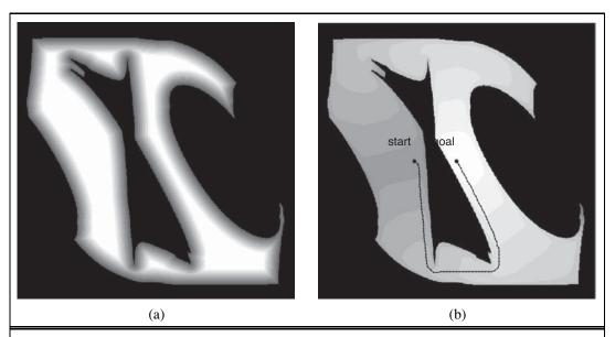
**Figure 25.17** (a) A repelling potential field pushes the robot away from obstacles. (b) Path found by simultaneously minimizing path length and the potential.
