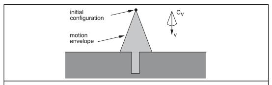
**Figure 25.19** A two-dimensional environment, velocity uncertainty cone, and envelope of possible robot motions. The intended velocity is v, but with uncertainty the actual velocity could be anywhere in  $C_v$ , resulting in a final configuration somewhere in the motion envelope, which means we wouldn't know if we hit the hole or not.
