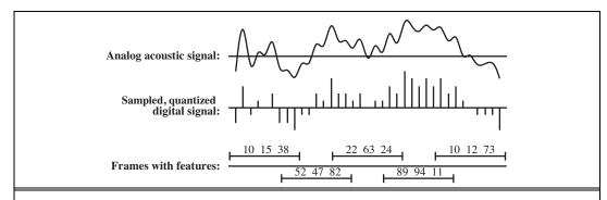
**Figure 23.15** Translating the acoustic signal into a sequence of frames. In this diagram each frame is described by the discretized values of three acoustic features; a real system would have dozens of features.
