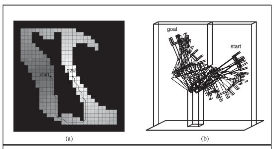
**Figure 25.16** (a) Value function and path found for a discrete grid cell approximation of the configuration space. (b) The same path visualized in workspace coordinates. Notice how the robot bends its elbow to avoid a collision with the vertical obstacle.
