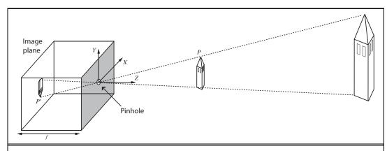
**Figure 24.2** Each light-sensitive element in the image plane at the back of a pinhole camera receives light from a the small range of directions that passes through the pinhole. If the pinhole is small enough, the result is a focused image at the back of the pinhole. The process of projection means that large, distant objects look the same as smaller, nearby objects. Note that the image is projected upside down.
