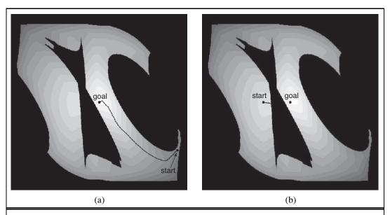
**Figure 25.23** Potential field control. The robot ascends a potential field composed of repelling forces asserted from the obstacles and an attracting force that corresponds to the goal configuration. (a) Successful path. (b) Local optimum.
