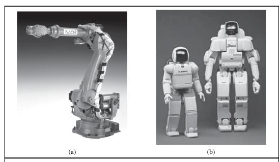
**Figure 25.1** (a) An industrial robotic manipulator for stacking bags on a pallet. Image courtesy of Nachi Robotic Systems. (b) Honda's P3 and Asimo humanoid robots.
