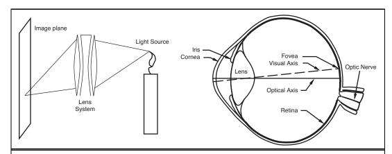
**Figure 24.3** Lenses collect the light leaving a scene point in a range of directions, and steer it all to arrive at a single point on the image plane. Focusing works for points lying close to a focal plane in space; other points will not be focused properly. In cameras, elements of the lens system move to change the focal plane, whereas in the eye, the shape of the lens is changed by specialized muscles.
