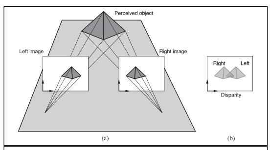
**Figure 24.16** Translating a camera parallel to the image plane causes image features to move in the camera plane. The disparity in positions that results is a cue to depth. If we superimpose left and right image, as in (b), we see the disparity.
