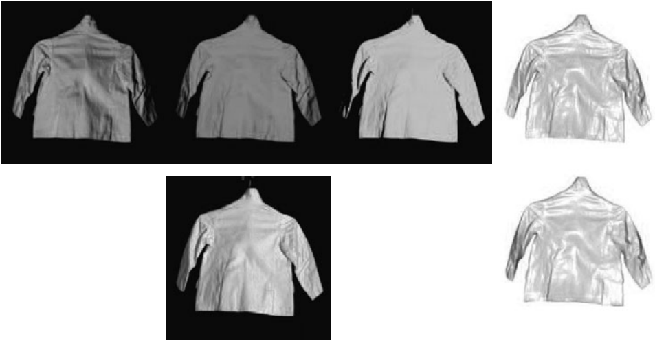
FIGURE 2.13: Photometric stereo could become the method of choice to capture complex deformable surfaces. On the top , three images of a garment, lit from different directions, which produce the reconstruction shown on the top right . A natural way to obtain three different images at the same time is to use a color camera; if one has a red light, a green light, and a blue light, then a single color image frame can be treated as three images under three separate lights. On the bottom , an image of the garment captured in this way, which results in the photometric stereo reconstruction on the bottom right . This figure was originally published as Figure 6 of “Video Normals from Colored Lights,” G. J. Brostow, C. Hernández, G. Vogiatzis, B. Stenger, and R. Cipolla, IEEE Transactions on Pattern Analysis and Machine Intelligence, 2011 © IEEE, 2011.
