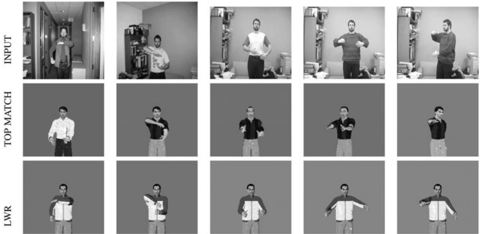
FIGURE 20.12: The 3D configuration of the body can be reconstructed using a form of nonparametric regression. Shakhnarovich et al. (2003) match the input frame ( top row ) to a large selection of labeled frames. The nearest neighbors are shown in the center row ; these give a fair reconstruction in most cases, but can be improved by finding multiple nearest neighbors and building a robust linear regression ( bottom row ). This figure was originally published as Figure 5 of “Fast Pose Estimation with Parameter-Sensitive Hashing,” by G. Shakhnarovich, P. Viola, and T. Darrell, Proc. CVPR 2003, 2003. © IEEE, 2003.
