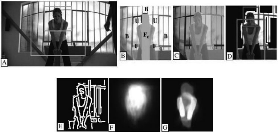
FIGURE 20.5: The human parser of Ramanan (2006) is a search of all spatial layouts in the image to find one that is consistent with the constraints we know on appearance. Ferrari et al. (2008) show that reducing the search space improves the results. First, one finds upper bodies, and builds a box around those detections using constraints on the body size (A). Outside this box is background, and some pixels inside this box are, too. In B, body constraints mean that pixels labeled F_c and F are very likely foreground, U are unknown, and B are very likely background. One then builds color models for foreground and background using this information, then uses an interactive segmenter to segment, requiring that F_c pixels be foreground, to get C. The result is a much reduced search domain for the human parser, which starts using an edge map D, to get an initial parse E, and, after iterating, produces F. This figure was originally published as Figure 2 of “Progressive search space reduction for human pose estimation,” by V. Ferrari, M. Marín-Jiménez, and A. Zisserman, Proc. IEEE CVPR 2008, © IEEE 2003.
