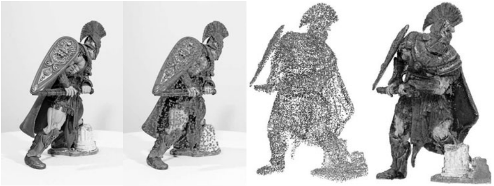
FIGURE 19.13: The PMVS approach to image-based modeling and rendering, illustrated using 48 1,800 \times 1,200 images of a Roman soldier action figure. From left to right: A sample input image; detected features; reconstructed patches after the initial matching; and final patches after expansion and filtering. Reprinted from “Accurate, Dense, and Robust Multi-View Stereopsis,” by Y. Furukawa and J. Ponce, IEEE Transactions on Pattern Analysis and Machine Intelligence , 32(8):1362–1376, (2010). © 2010 IEEE.
