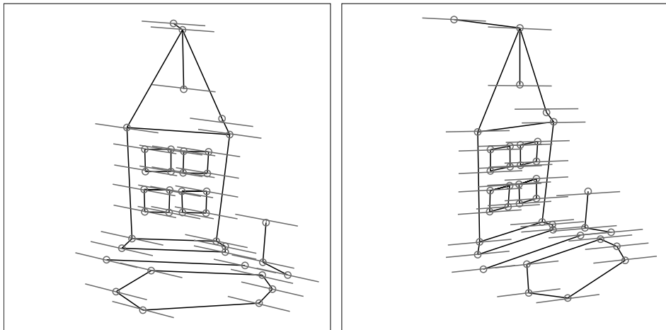
FIGURE 8.2: Weak-calibration experiment using two images of the house sequence and a linear least-squares implementation of weak calibration, together with Hartley’s normalization. The mean distances between the points and the corresponding epipolar lines are 0.96 and 0.90 pixels for these two images. Without the normalization, they become 10.00 and 9.12 pixels.
