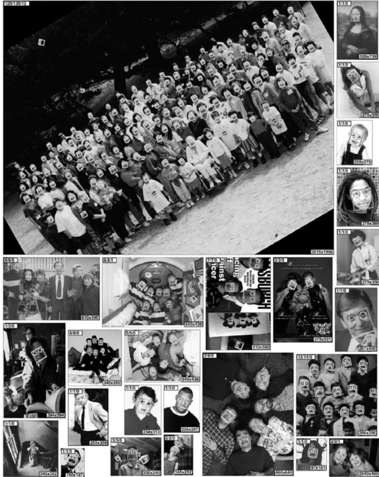
FIGURE 17.3: Typical responses for the Rowley, Baluja, and Kanade system for face finding; a mask icon is superimposed on each window that is determined to contain a face. The orientation of the face is indicated by the configuration of the eye holes in the mask. This figure was originally published as Figure 7 from “Rotation invariant neural-network based face detection,” H.A. Rowley, S. Baluja, and T. Kanade, Proc. IEEE CVPR, 1998, © IEEE, 1998.
