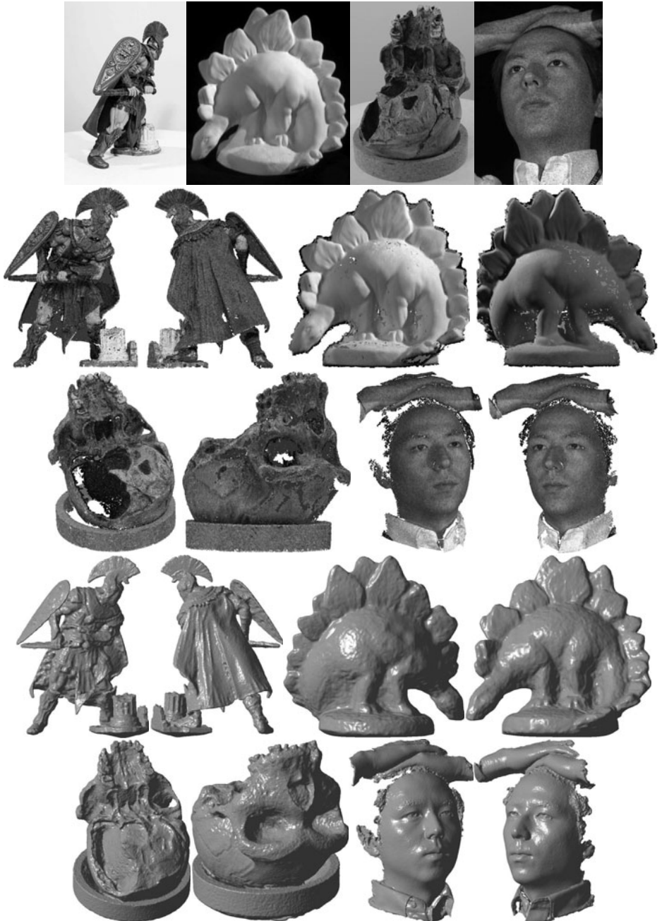
FIGURE 19.19: From top to bottom : Sample input images, reconstructed patches, and final mesh models. Reprinted from “Accurate, Dense, and Robust Multi-View Stereopsis,” by Y. Furukawa and J. Ponce, IEEE Transactions on Pattern Analysis and Machine Intelligence , 32(8):1362–1376, (2010). © 2010 IEEE.
