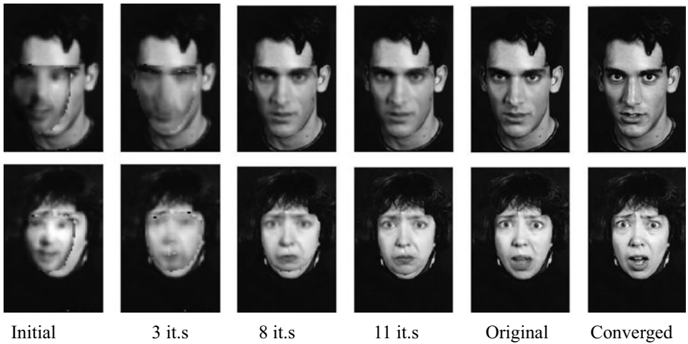
FIGURE 12.10: Active appearance models registered to face images. On the left , the initial configuration of the model (blurry blob over the face; original face is second from right). As the minimization process proceeds, the search improves the registration to produce, in the final converged state, the registration on the right . Once we have this registration, the location of the vertices of the mesh and the deformation parameters encode the shape of the face. This figure was originally published as Figure 5 of “Active Appearance Models,” by T. Cootes, G. Edwards, and C. Taylor, IEEE Transactions on Pattern Analysis and Machine Intelligence, 2001, © IEEE, 2001.
