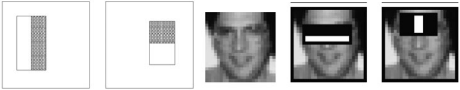
FIGURE 17.4: Face detection can be made extremely fast using features that are easy to evaluate, and that can reject most windows early. On the left , features can be built up out of sums of the image within boxes, weighted by 1 or -1 . The drawings show two two-box features (some readers might spot a relationship to Haar wavelets). On the right , the features used for the first two tests (equivalently, the first two classifiers in the cascade) by Viola and Jones (2001). Notice how they check for the distinctive dark bar at the eyes with the lighter bar at the cheekbones, then the equally distinctive vertical specularly along the nose and forehead. This figure was originally published as Figures 1 and 3 from “Rapid Object Detection using a Boosted Cascade of Simple Features,” by P. Viola and M. Jones, Proc. IEEE CVPR 2001 © IEEE 2001.
