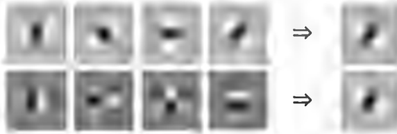
Figure 19.6 Two different sets of basis functions can be used for the construction of a steered Gaussian derivative kernel. Upper row: the basis set is formed from rotated versions of the kernel itself; bottom row: the basis set is formed from Cartesian x, y -separable Gaussian derivative kernels. The weights are calculated in the section above. Kernel as in figure 19.5.
