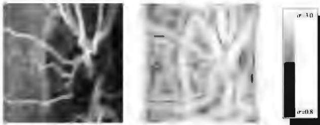
Figure 17.12 Left: eighth frame of the image sequence. Right: scale index for the maximum singular value of the coefficient matrix of the optic flow equations, for the scale range \sigma = 0.8 to 3 pixels. Note the smaller scales for the locations rich with image structure, such as the vessels, and the use of larger scales for the more homogeneous areas.
