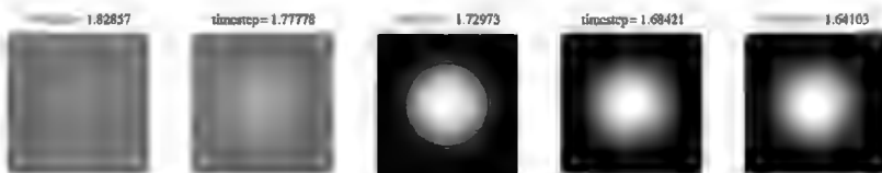
Figure 21.13 Study of the influence of time stepsize on the accuracy of the result in the numerical approximation of the linear diffusion equation. Image resolution 128^2 , evolution to s = 64 pixel 2 , scale Laplacian operator \sigma = 0.8 pixel. The critical timestep \Delta s = e \sigma^2 = 2.1718 \times 0.8^2 = 1.74 .
