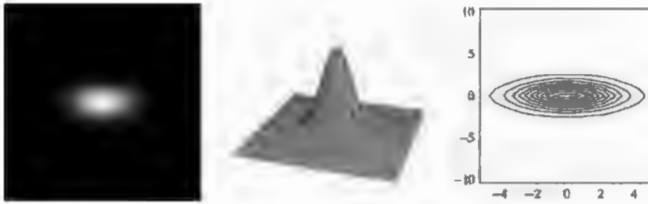
Figure 3.16 An anisotropic Gaussian kernel with anisotropy ratio \sigma_x/\sigma_y=2 in three appearances. Left: DensityPlot , middle: Plot3D , right: ContourPlot .
